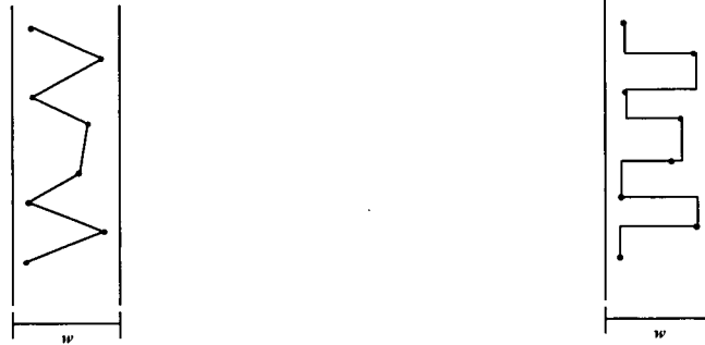
a) Euclidiana d = [(x_B - x_A)^2 + (y_B - y_A)^2]^{1/2} b) Retangular d = |x_B - x_A| + |y_B - y_A|
