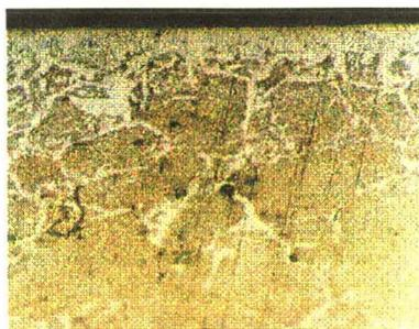
Fig. 5a. Plasma-surface interaction in Ar-O<sub>2</sub>. Decarburization process is shown on top surface of AISI 1045 sample.
