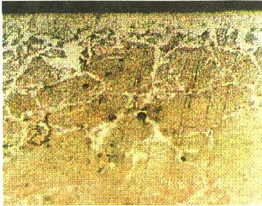
Fig. 2a. Plasma-surface interaction in Ar-O<sub>2</sub>. Decarburization process is shown on top surface of AISI 1045 sample.
