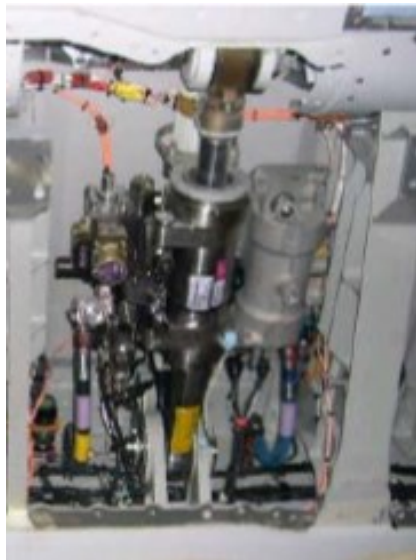
Figure 3.2 - Airbus A380 Servo Hydraulic Actuator.
