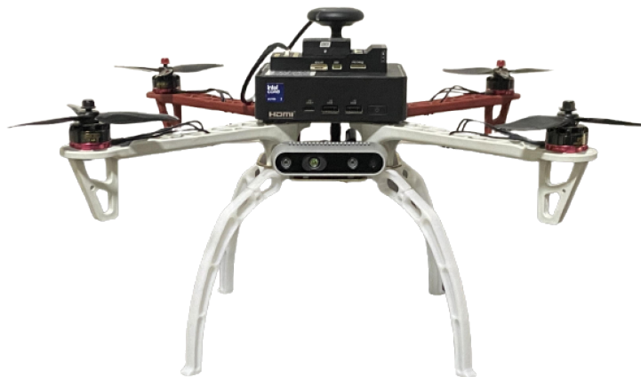
Figure 23 – Drone Hardware Prototype.
