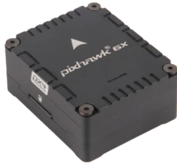
Figure 8 – Holybro Pixhawk 6X model.
