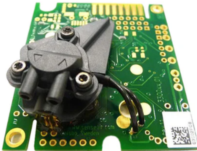
Figura 3 – K33 CO 2 Sensor SenseAir.
