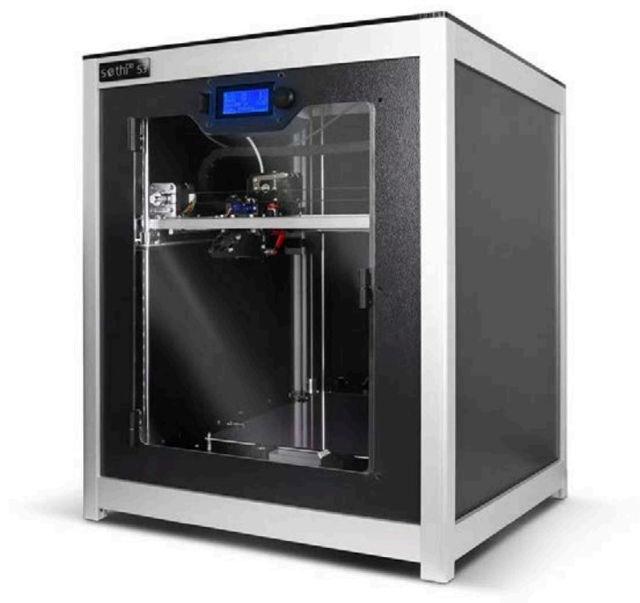
Figura 84: Impressora FDM Sethi3D S3
