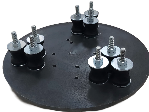
Figure 25 – Circular steel plate with nine bushings attached to it.
