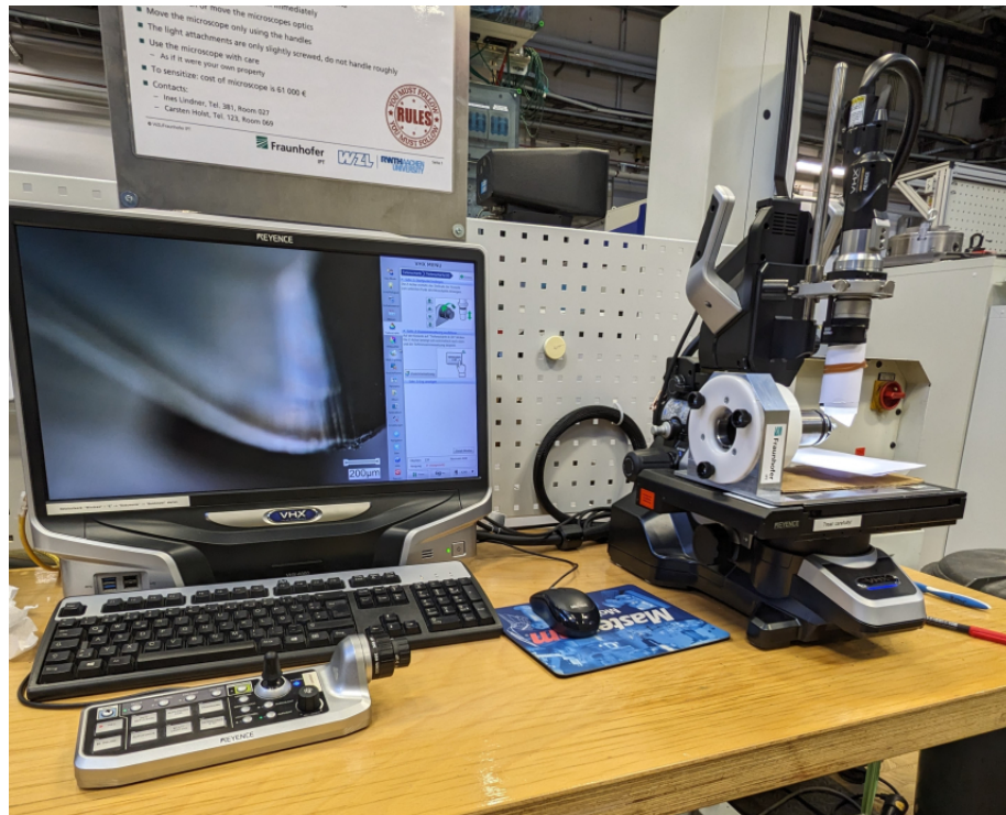
Figure 36 – Digital microscope for image acquisition of cutting edges, chips and machined surface
