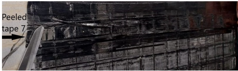
Figure 35 – Peeled tape 7 on first laminate.
