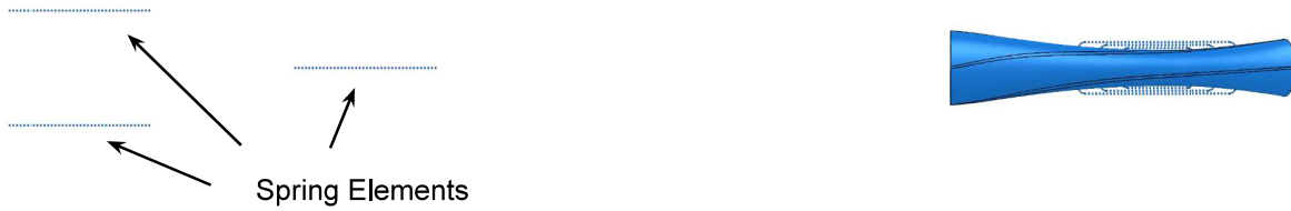
Figure 12 – Detail of the position of the spring elements representing the muscle passive stiffness.
