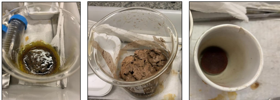
Figure 4. Synthesis Steps of LaFeO 3 Perovskite.
