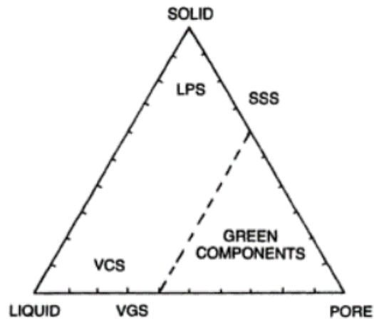
Figure 2.3: Ternary solid-liquid-pore diagram showing different types of sintering.
