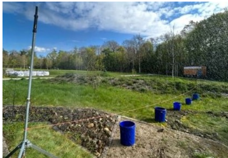
Figure 22 – Evaluation of Sprinkler's performance
