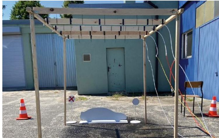
Figure 14 – Outdoor Ring for rain generation
