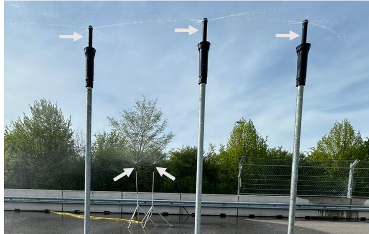
Figure 24 – Sprinklers positioned in the outdoor facility for the rain of 25 mm/h, lateral view
