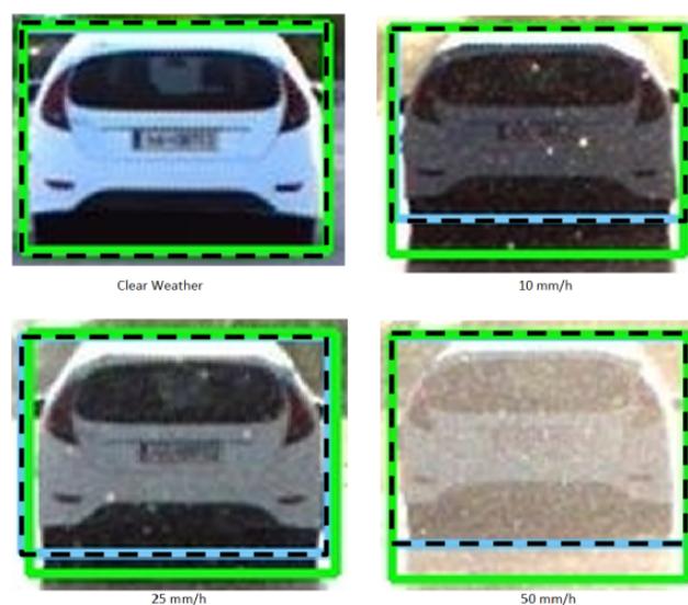
Figure 49 – Detection frames for the three rain intensities for the position target of 28 m
