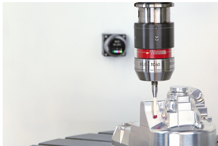
Figure 31 – Touch probe measuring a workpiece.
