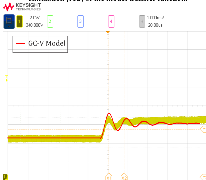
Figure 4.4 – Duty cycle step response of the GC-V prototype (yellow) versus PSIM simulation (red) of the model transfer function.
