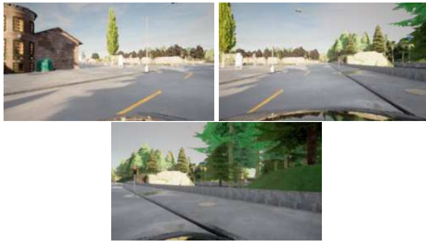
Figure 4 – Images from the three frontal cameras located at the left, central, and right part of the vehicle, respectively. They were taken after the first few interactions of the agent in the CARLA simulation environment considering our defined trajectory. Each camera produces a RGB image with 144 pixels of height and 256 pixels of width. These images are fed to the networks as they are.
