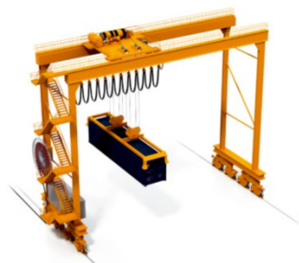
Figura 13 - Automated Stacking Cranes (ASC)
