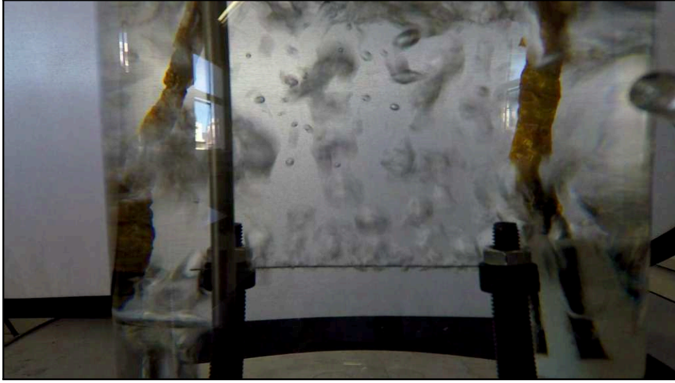
Figure 16 – Example video frame obtained at 75 W for the baseline, large wire dataset \mathcal{D}^{LW} . The video frame contains environmental clues such as the LED or reflexes, which are cropped out of the ROI, as described in Section 4.2.2.
