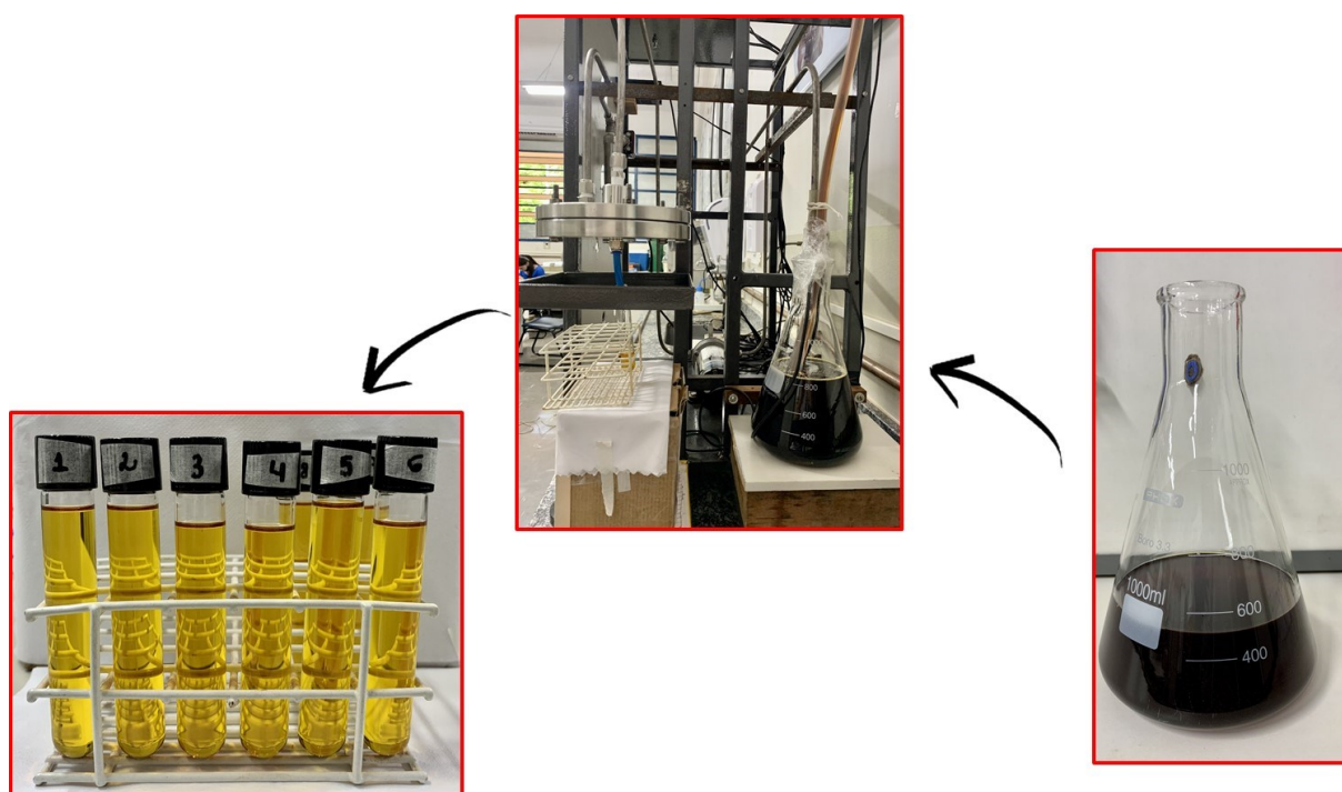
Figure 34. Schematic representation of the steps for obtaining permeates from the industrial sample.
