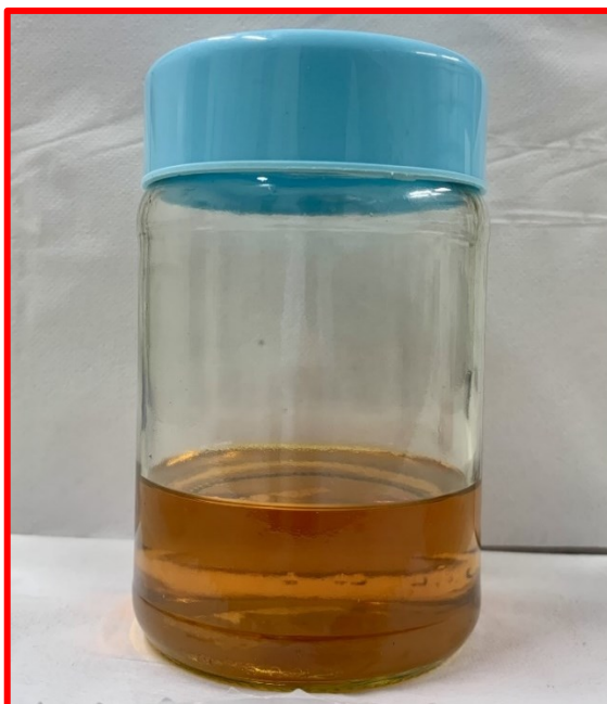
Figure 38. Fatty acid methyl ester obtained after polishing through UF with 10 kDa PES membrane.
