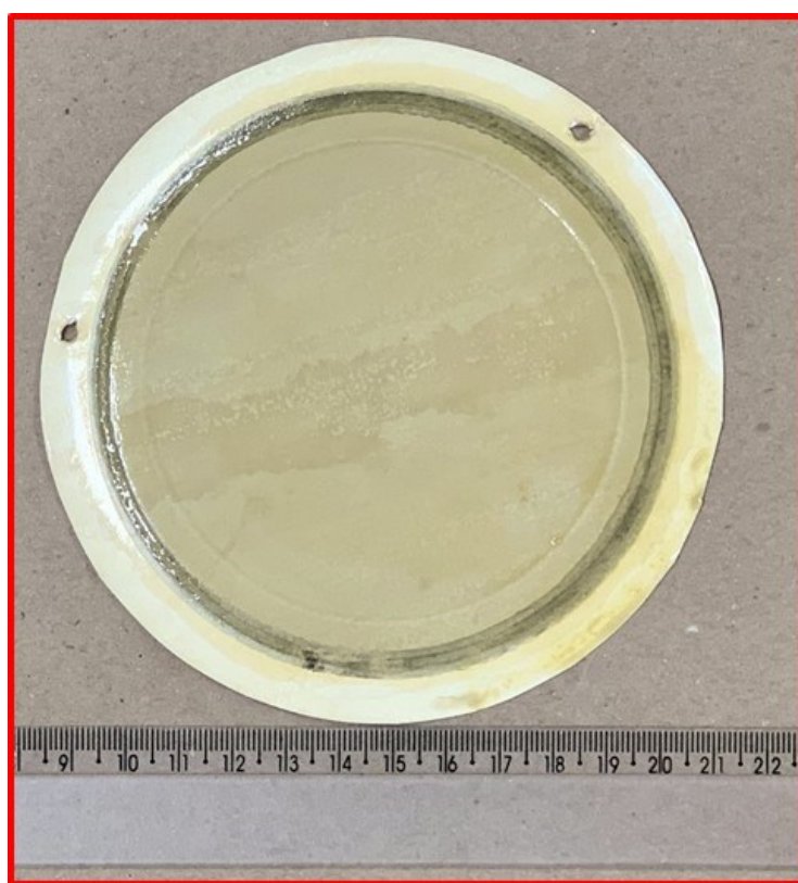
Figure 26. Surface NF-90 membrane after contact with industrial FAME in separation attempt.
