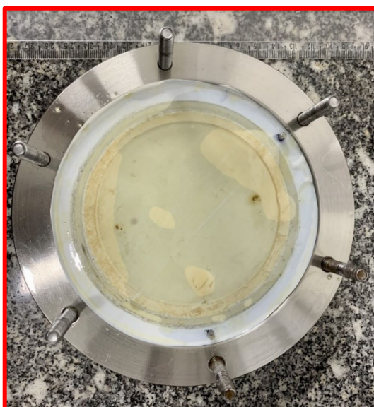
Figure 36. Membrane surface after direct contact with real industrial FAME for 70 h in a crossflow filtration system at 3 bar.
