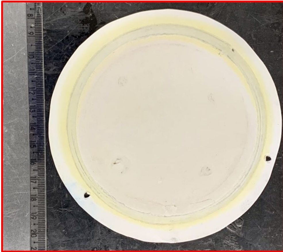
Figure 21. PVDF Membrane surface after permeation tests with “on spec” biodiesel.
