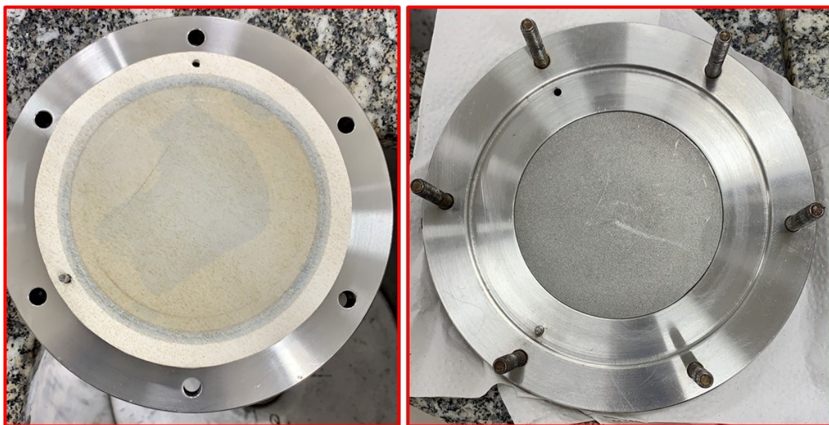
Figure 25. Dry membrane module after filtration test.
