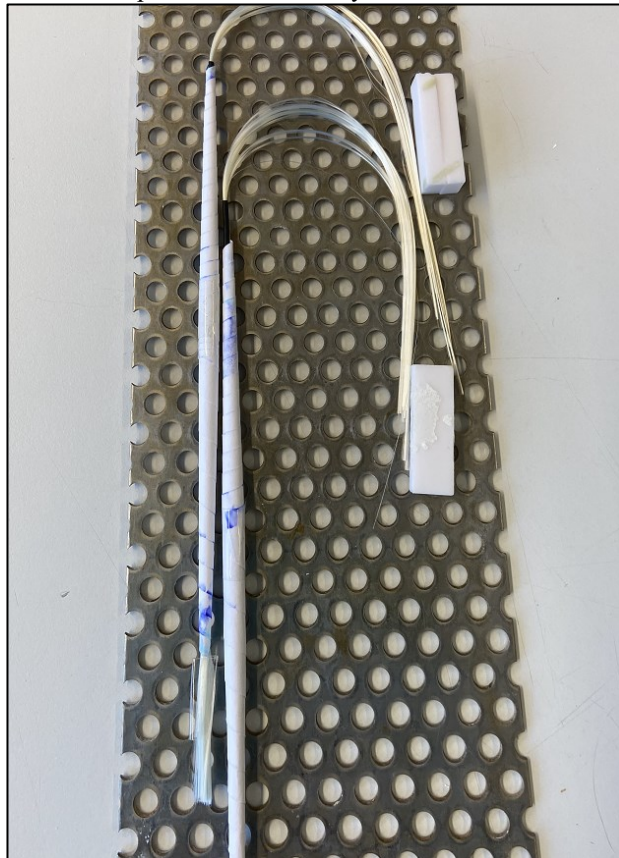
Figure 25 – Minicomposite sample preparation. In this step, fibers were being prepared for plasma deposition previous to the slurry infiltration.
