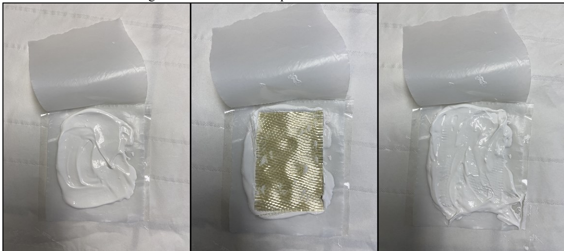
Figure 29 – Infiltration steps done on ceramic fabrics.
