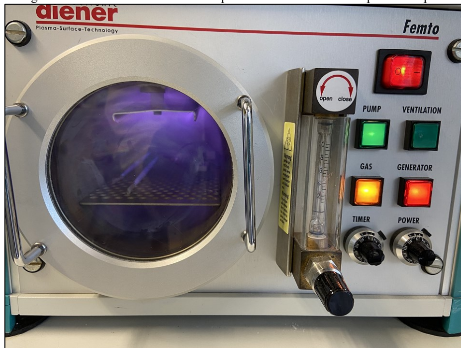
Figure 14 – Plasma surface treatment performed on fibers of composite samples.
