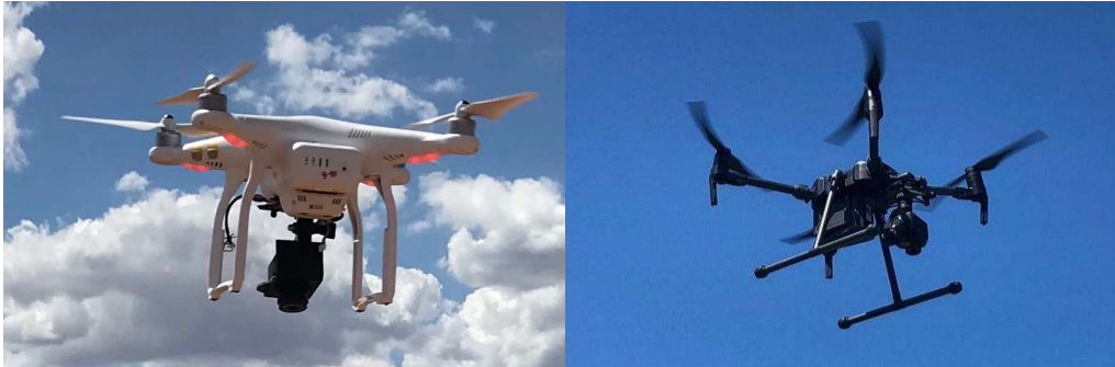
Figure 3-2 - aIRT measurement systems applied with extra lightweight IRT camera adapted to commercial drone (System 1 (left) in Table 3-1, and high-end, fully commercial IRT+RGB drone System 2 (right) in Table 3-1).
