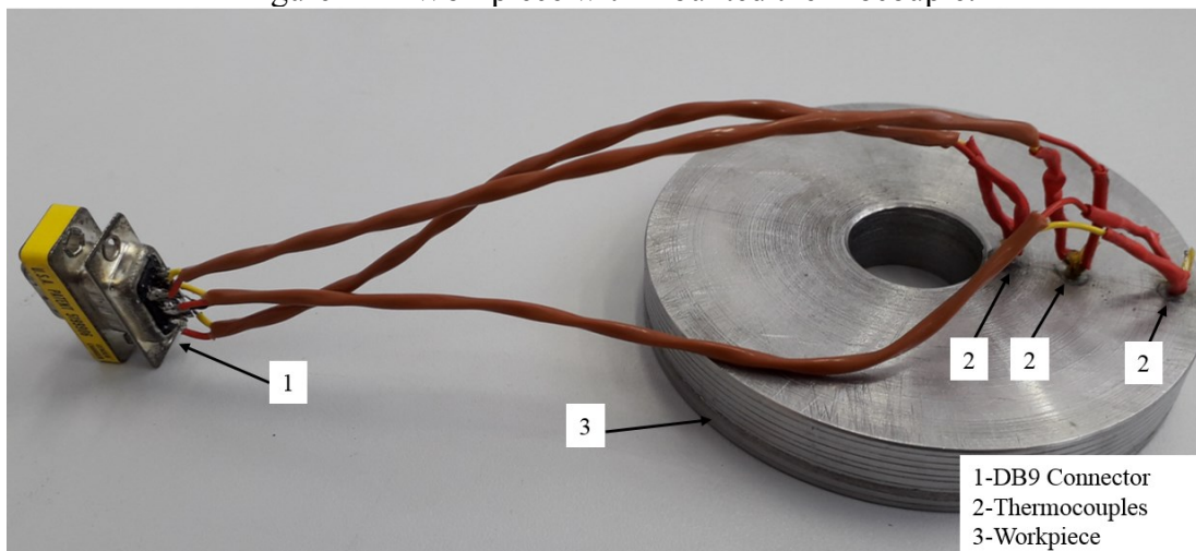
Figure 42 – Workpiece with mounted thermocouple.
