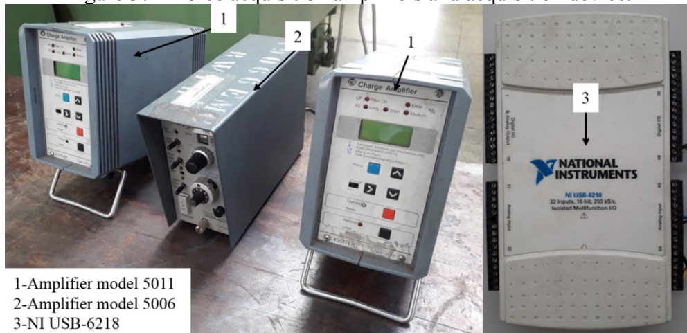
Figure 37 – Force acquisition amplifiers and acquisition device.
