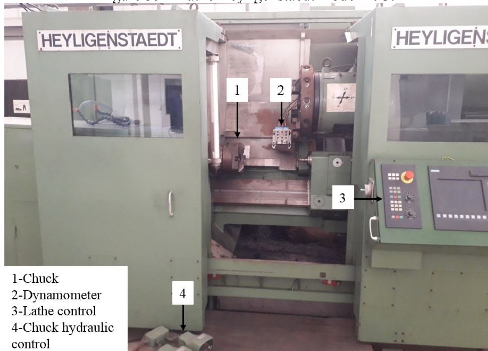
Figure 35 – Lathe Heyligenstaedt model 10U.
