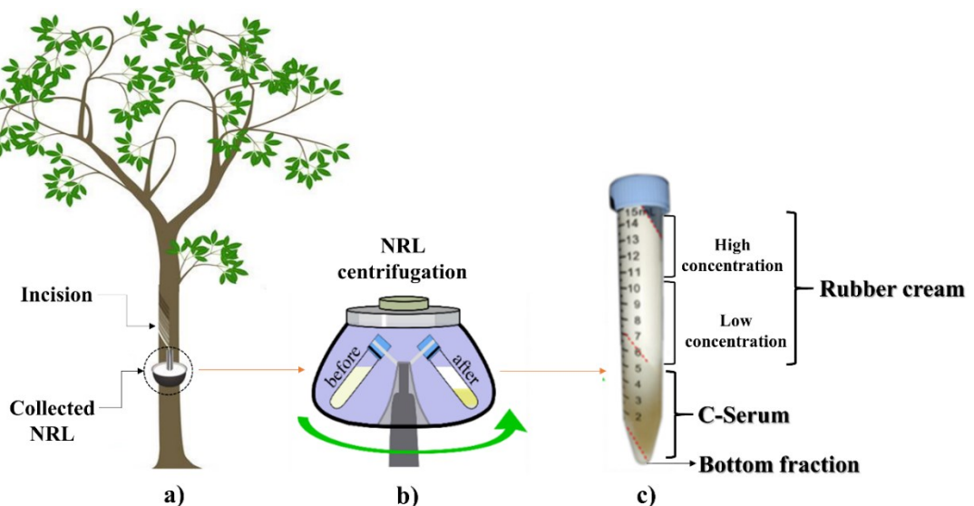
Figure 4 - Natural rubber tapping for collection of latex, b) centrifugation process and c) separation of latex into different phases after centrifugation.
