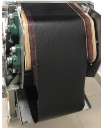
Figure 21 - Detachment of the dried açai-pectin suspension from the conveyor belt.
