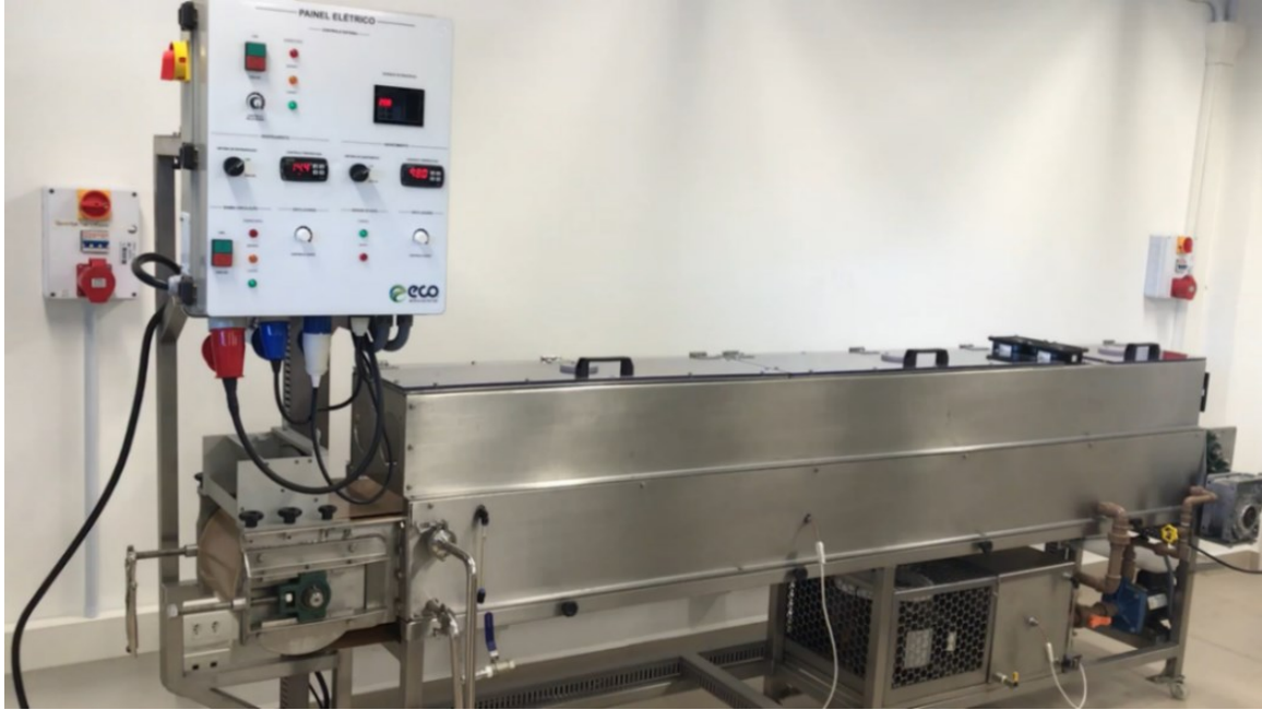
Figure 17 - Device of the continuous cast-tape drying.
