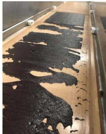
Figure 19 - Spreading of the açai juice-pregelatinized starch suspension.
