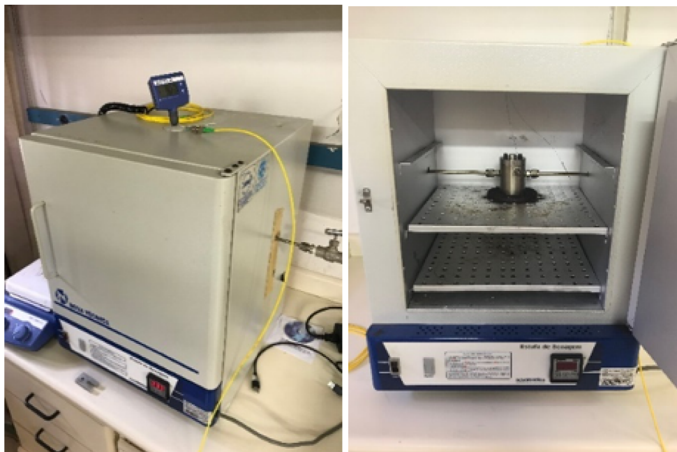
(a) Stove closed and the termocouple PT100 used for the calibration. (b) Stove with the FBG temperature sensor positioned inside.
