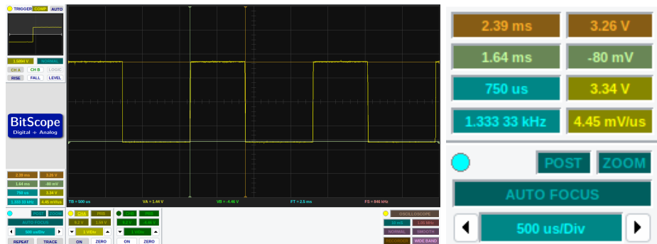
Figure 16 – Oscilloscope image of a GPIO toggle with the FFT and peak calculation in between.
