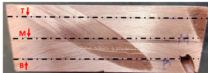
Figure 14 – Top (T), middle (M) and bottom (B) parts of interest to verify homogeneity and presence of pores of the samples from the casting.
