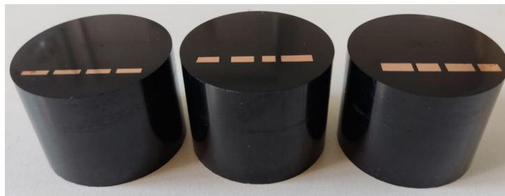
Figure 21 – Final aspect of the metallographic preparation for optical microscopy analysis after laser ultrashort ablation.
