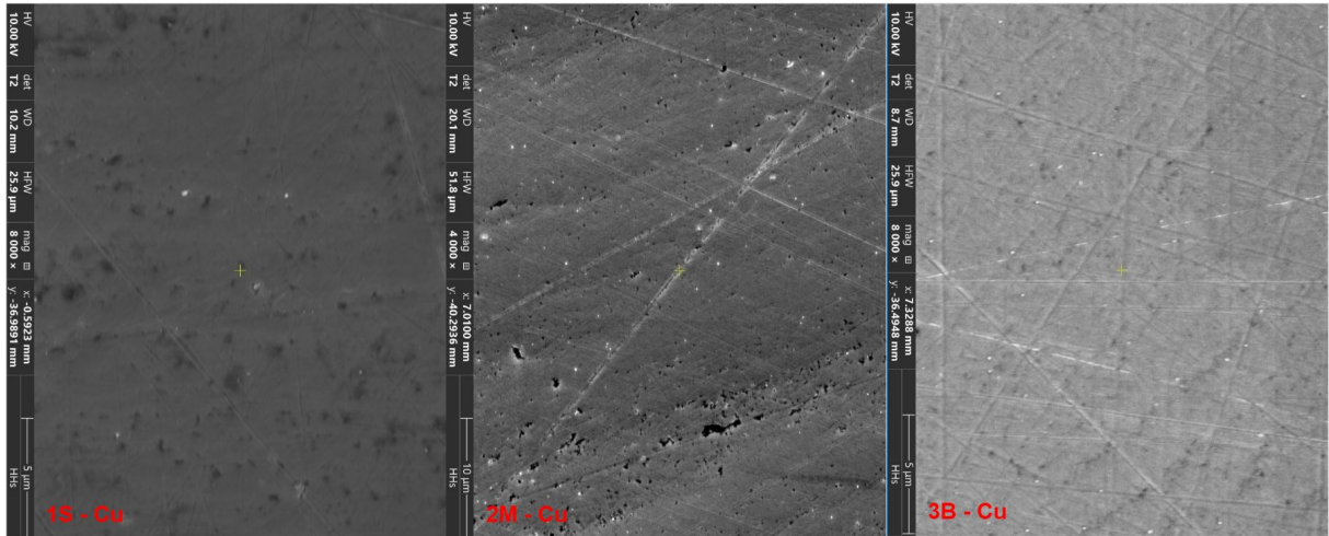
Figure 27 – Original copper surface without ablation marks of samples 1S, 2M and 3B.
