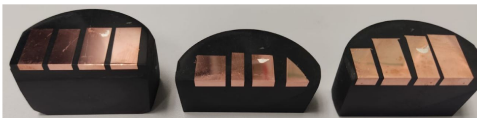
Figure 17 – Cut and polished samples ready for the ultra-short laser ablation process.
