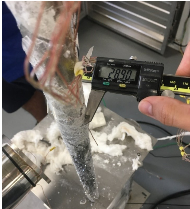
Figure 5.13. Picture from the evaporator after removal from 1\frac{1}{4} " PCM container, from Test 6 (Table 3.4), with a digital caliper measuring the solidified layer thickness at one of the points where it was intact.
