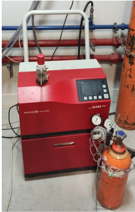
Figure 3.4. Helium leak detector, Pfeiffer Vacuum ASM 340.
