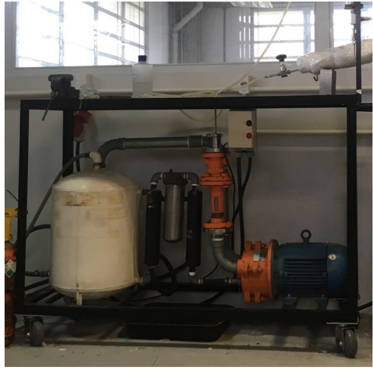
Figure 3.5. Closed two-phase thermosyphon being evacuated by a liquid ring vacuum pump.
