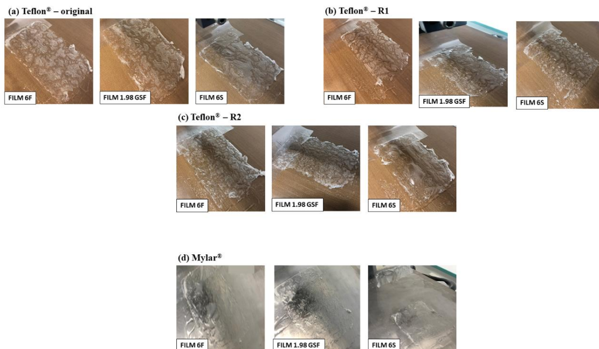
Figure 41 - Starch-based films formed over (a) Teflon ® ; (b) Teflon ® R1; (c) Teflon ® R2 and (d) Mylar ® .
