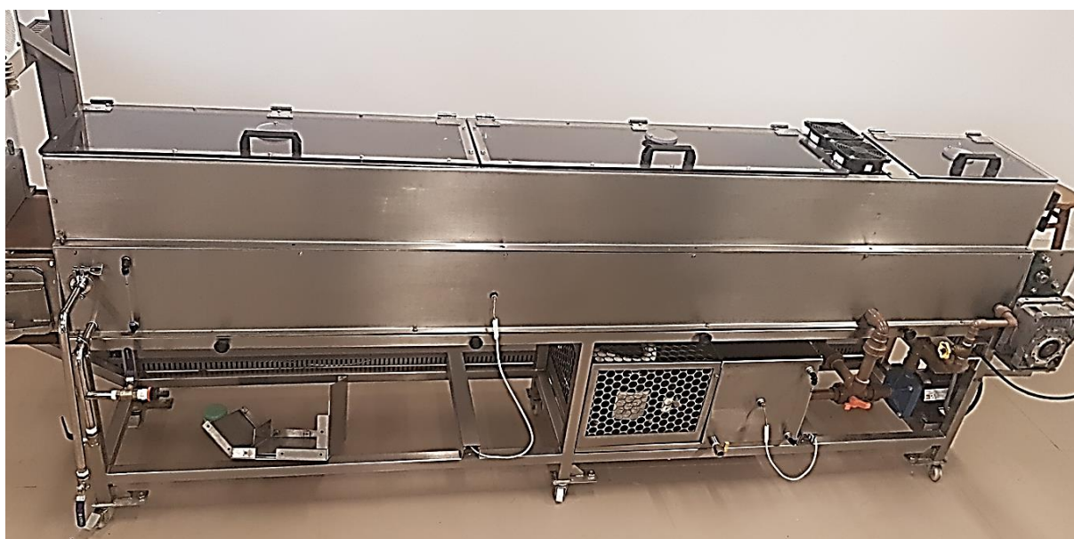
Figure 12 - Image of the continuous CTD equipment used in the experiments.
