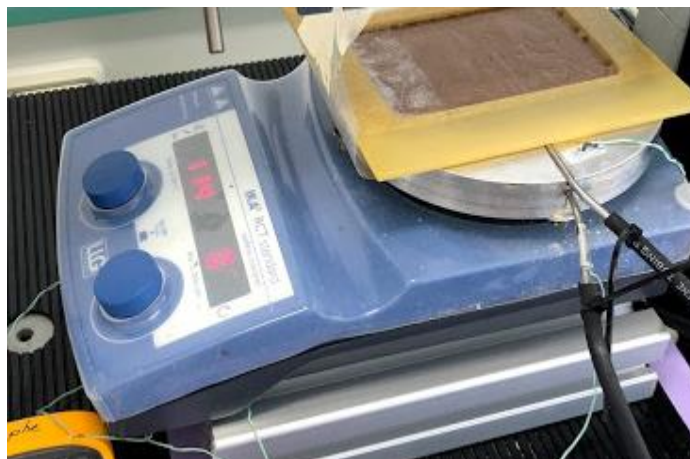
Figure 19 - Aluminum plate employed to detachment tests with cooling.
