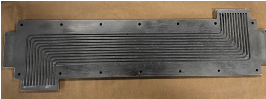
Figure 43 – Heat exchanger core showing side with channels of square cross-section.
