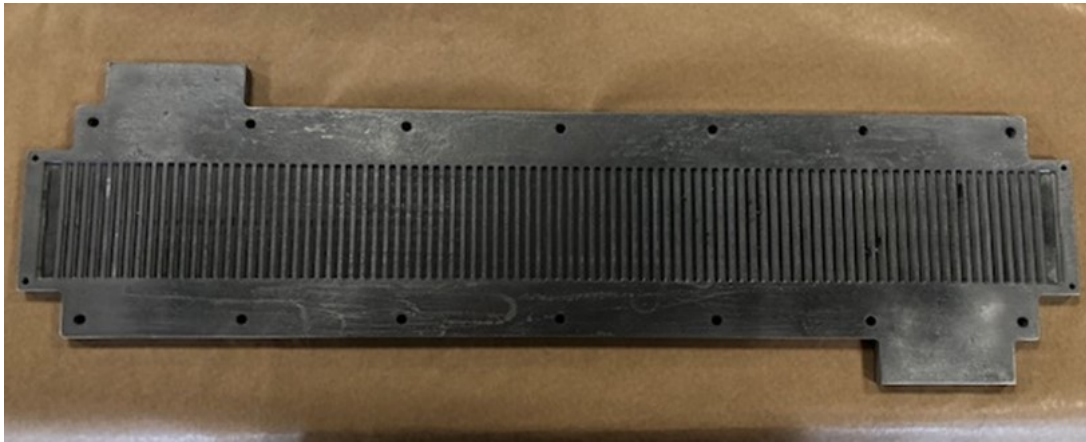
Figure 43 – Heat exchanger core showing side with channels of square cross-section.
