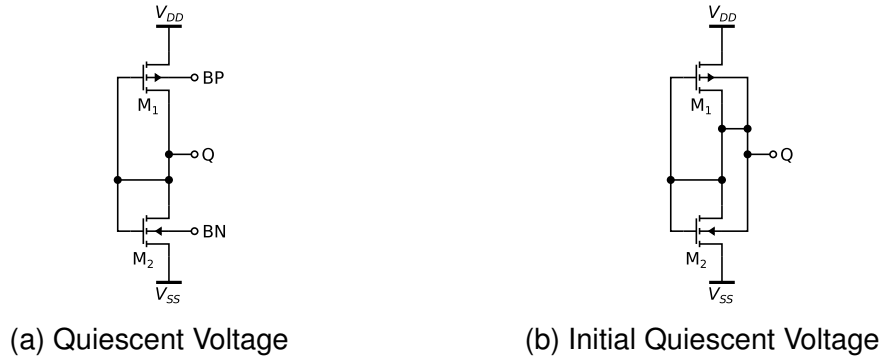
Figure 51 – Quiescent Voltage Extraction Circuits
