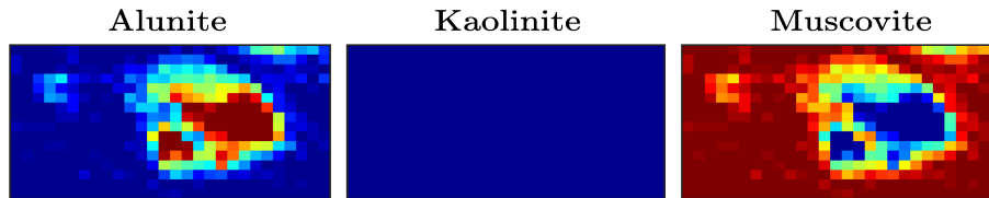
Figure 42 – Abundance maps of MESMA for the Alunite Hill HI with a spectral library augmented using the Hapke model with known acquisition conditions.
