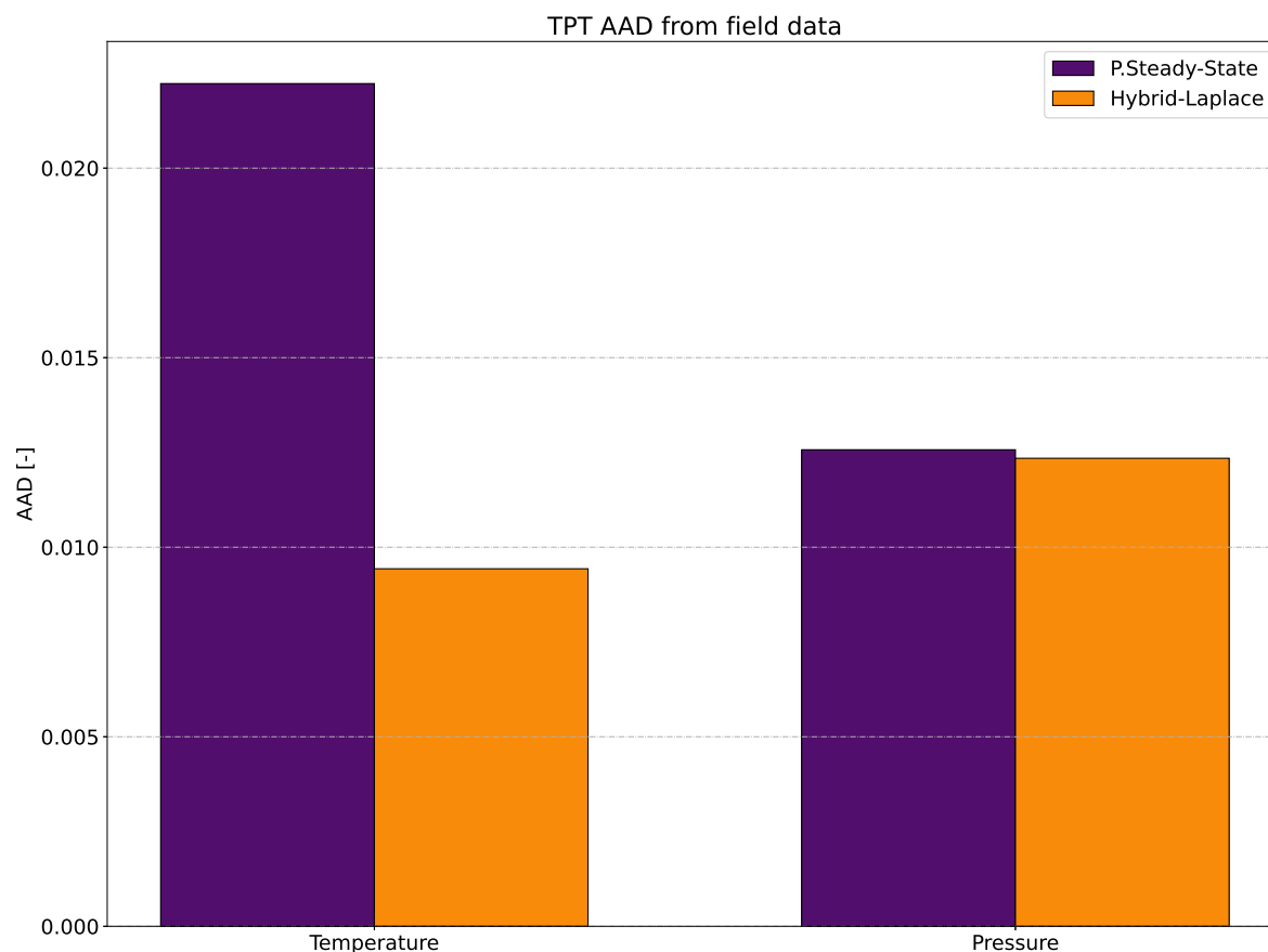
Figure 67 – AAD from temperature and pressure at the TPT for the EWT well
