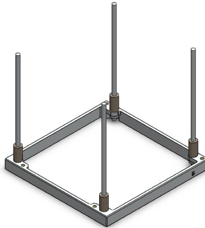
Figure A.19: Ring B + rods + spacers.
