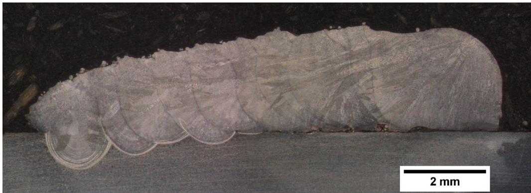
Figure 61 – Cross-section of deposition with high layer slope and decreasing dilution due to low hatch spacing (the deposition starts from the left).
