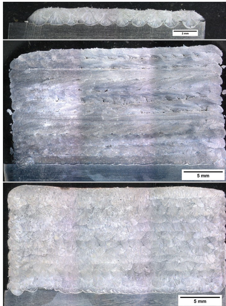
Figure 68 – Verification of the predicted single-layer (a) and the blocks using 5% (b), 10% (c), 15% (d), 20% (e), and 25% (f) of overlayer.
