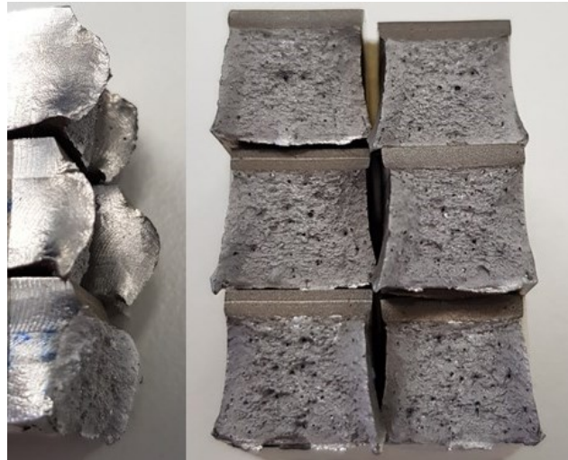
Figure 88 – Ductile fracture of the impact absorption samples.
