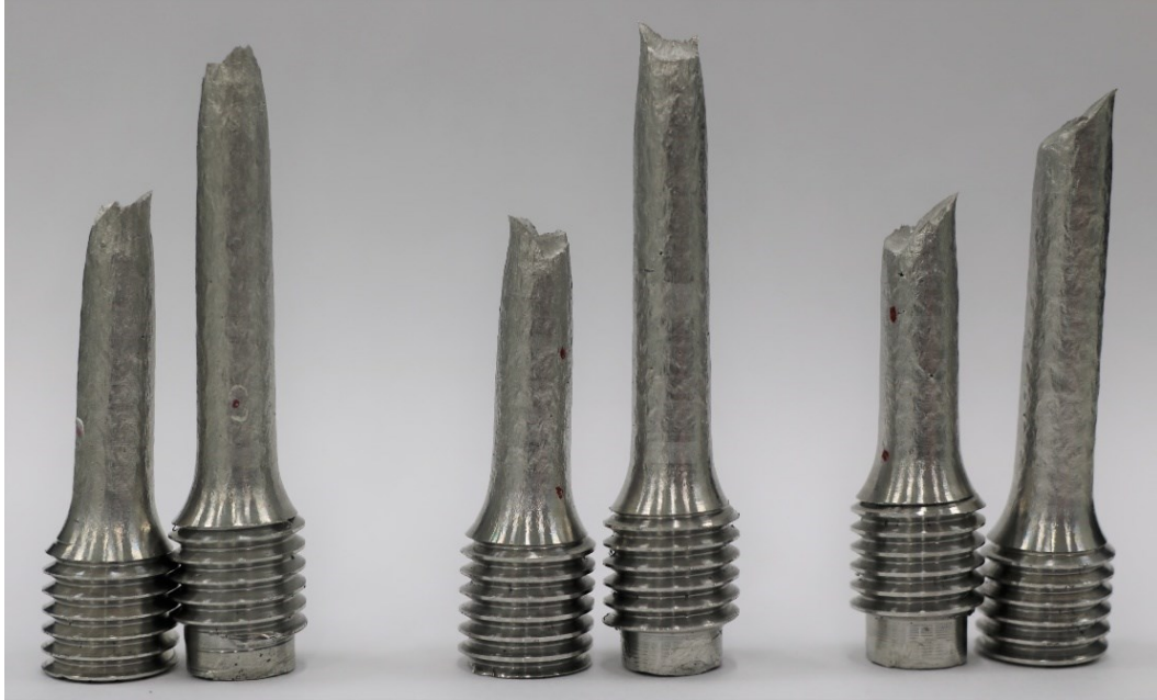
Figure 86 – Vertical HT sample T1V-1 (left), vertical AB sample T2V-3 (center), and vertical AB sample T1V-3 (right) showing the shape of the fracture after the tensile test. Only the right sample exhibits brittle behavior.
