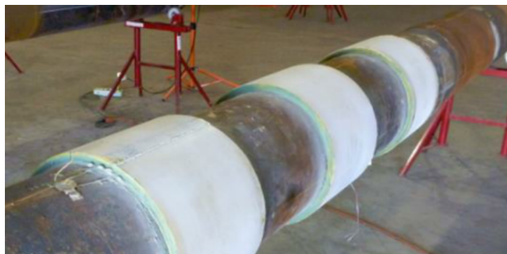
Figure 36 – A pipeline sample with its three composite repairs (FRÖHLICH et al., 2018).
