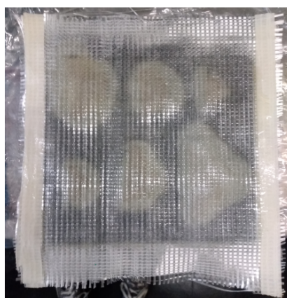
Figure 44 – Left: SCT-plate with semi-circular after lamination. Right: after it has been housed in a sealed bag and vacuum has been induced.
