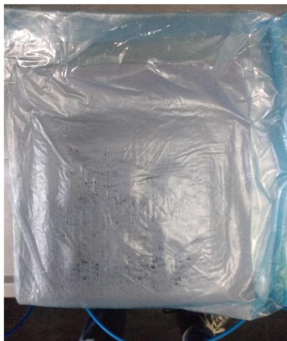
Figure 44 – Left: SCT-plate with semi-circular after lamination. Right: after it has been housed in a sealed bag and vacuum has been induced.
