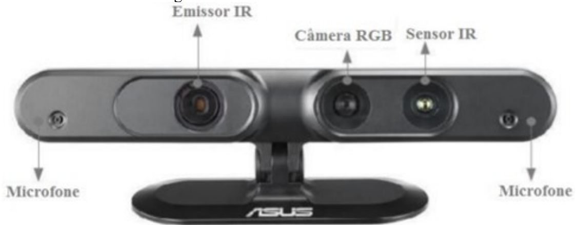
Figura 3.13 – Sensor Xtion PRO LIVE .
