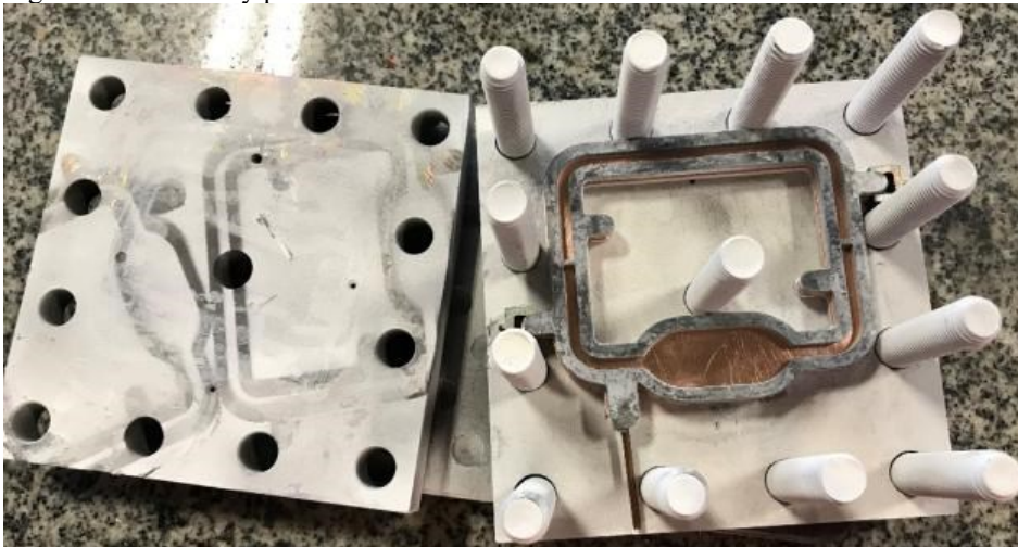
Figure 28 - Assembly process with the UTLHP and its matrix.
