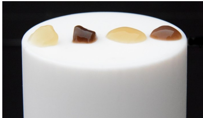
Figure 30 - Image of the \text{Ca}^{2+} -ALE samples with a controlled dry matter content of 2.3% (from left to right: AGS simple synthetic , AGS real , AGS complex synthetic and AS real ).
