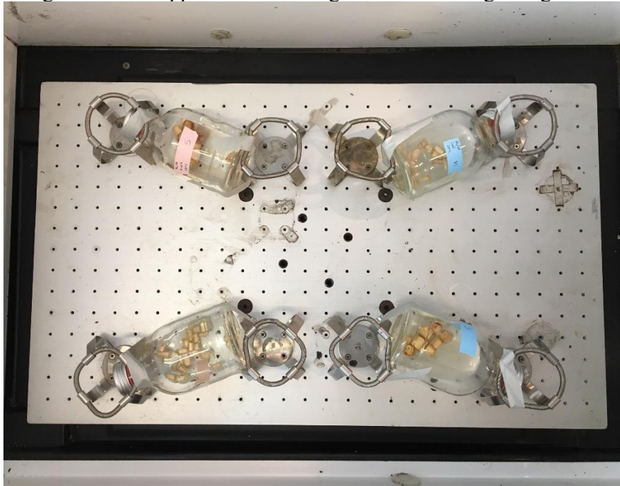
Figure 10 - PT applied to 1 cm length stems in the agitating oven.
