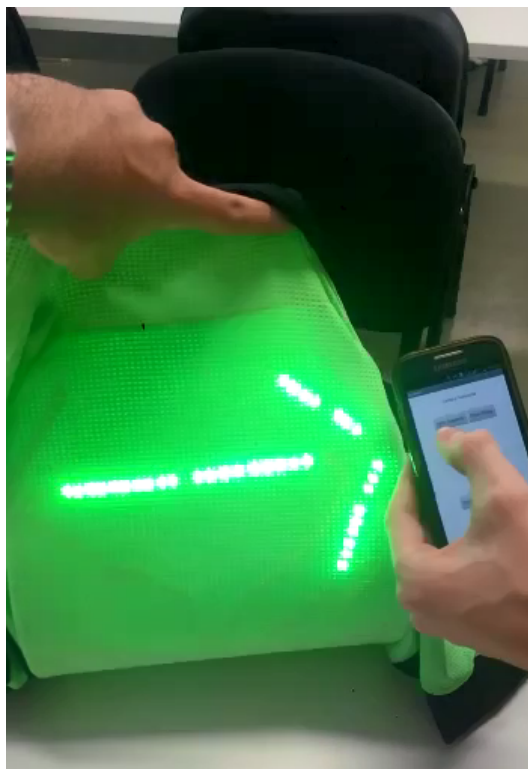
Figura 39 – Bluetooth acionando as setas de LEDS.
