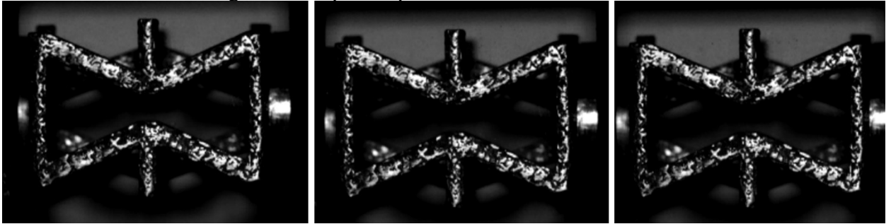
Figure 95 – Split-Hopkinson bar test of STR3.
