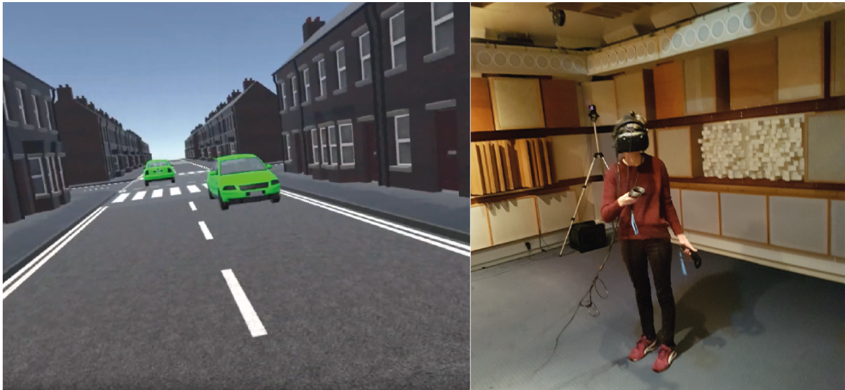
Figure 15 – Experiment 3: On the left side, the participant’s view of the environment. The green cars represent that the participant has already noticed them. On the right side, the participant located in the Listening Room.
