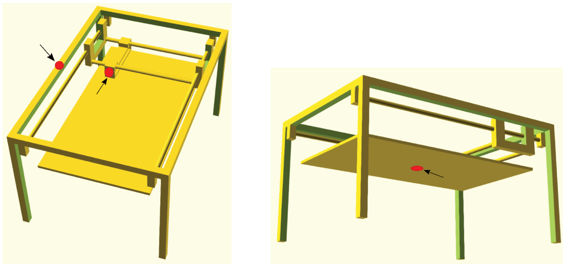
Figure 30 – INCANTO Project Printer Schema - Accelerometers’ installation.
