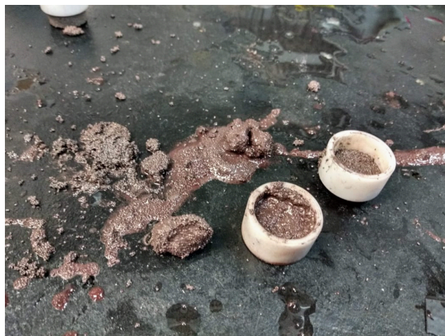
Figure 44 – Photograph of the opened cylindrical-pellet regenerator after being tested.
