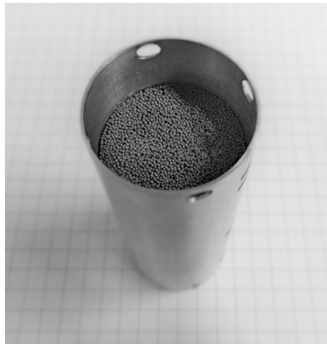
Figure 41 – Photograph of the bed of Regenerator-1 inside the AISI 304 stainless steel casing.
