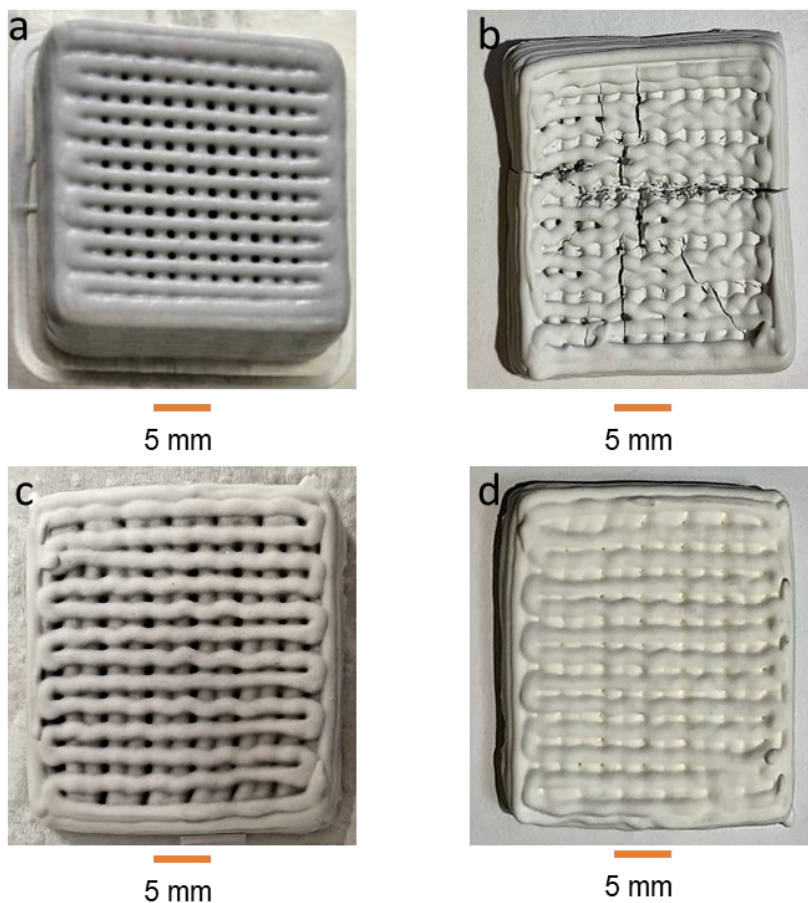
Figure 44 – Photograph showing 3D-printed sodium alginate samples. (a) right after shaping, (b) room temperature drying (c) freeze dried and (d) post firing final body.
