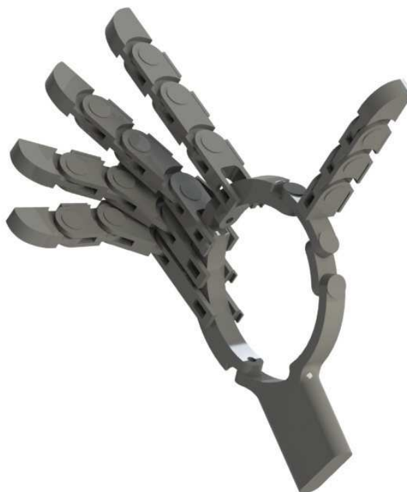
Figure 50 – CAD model of the anthropomorphic reconfigurable palm.
