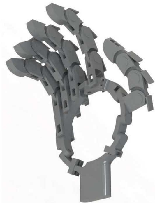
Figure 64 – New Self-Aligned Reconfigurable Anthropomorphic Hand
