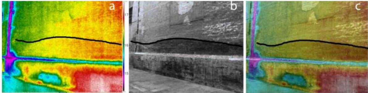
Figure 7 - Capillary rise of the water: (a) thermographic camera, (b) photographic camera and previous superposition images (c).
