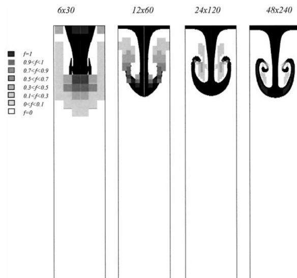
Figure 2.13 – Rayleigh-Taylor instability simulated through the VOF-TFM coupled method in different mesh resolutions t=2.0 s.
