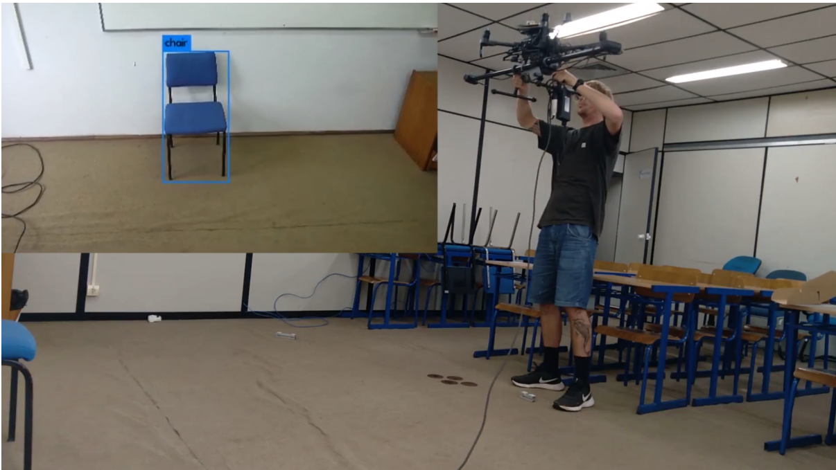
Figure 57 – RPA starting a vertical movement while tracking the object
