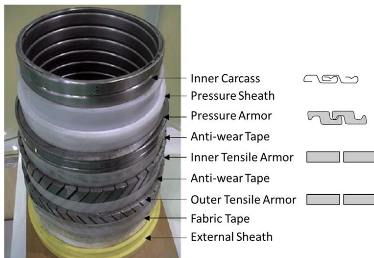
Figure 2 – Typical structure of flexible riser .
